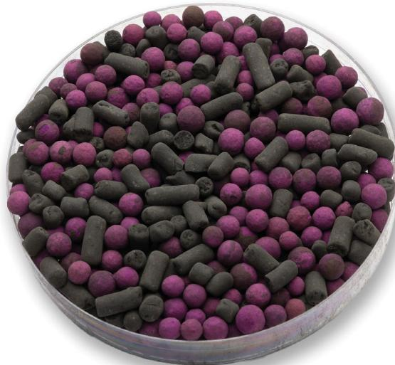
PureAir provided Spokane with Packed Bed Systems (PBS) equipped with two media beds for Sulphasorb XL™ and CPS Blend adsorbent media. Sizes custom engineered ranged from PBS-404 to PBS-809. The odors the project was designed to tackle were hydrogen sulfide, VOCs, mercaptans, and sulfur compounds.
