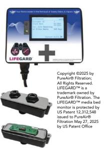
The Environment Corrosivity Monitor (ECMv2) detects corrosion in real time with live readings of airborne corrosivity.
