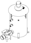
BLOWER-MOTOR ASSEMBLY MEDIA BED MONITORING ROD SAMPLE PORTS MEDIA BED #2 DIFFERENTIAL PRESSURE GAUGE MEDIA BED #1 MIST & GREASE -media bed Support platform DRAIN L1 ELEVATION VIEW
