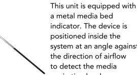
a metal media bed indicator. The device is positioned inside the system at an angle against the direction of airflow to detect the media expiration level.
