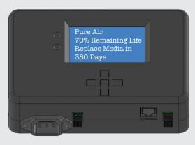
The EBMv2 now incorporates six externally wired and mounted sensors designed to detect variations in adsorbent media life. These sensors transmit data to the control panel, which utilizes a proprietary algorithm to predict the media consumption date.
